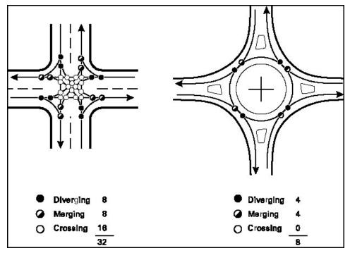
Figure 1. Comparison of vehicle-vehicle conflict points for four-legged intersection and roundabout (Robinson, Rodegerdts, Scarborough et al. 2000).
